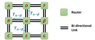
Figure 5: NoC with routers connected in a  $3 \times 3$  Mesh topology. Illustrative example showing that once a communication completes, the direct trust between  $\alpha$  and  $\beta$   $(T_{\alpha \to \beta})$  is delegated to nodes one hop away from  $\alpha$ .
