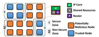
Figure 1: Overview of a typical SoC architecture with secure and non-secure zones.
