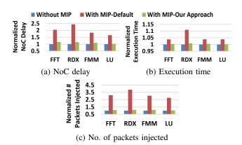
Figure 6: NoC delay, execution time and number of packets injected with and without our trust-aware routing model when running real benchmarks. p = 20 and n = 14. This figure is an extension of Figure 2.
