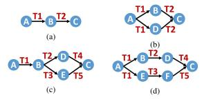
Figure 3: Trust delegation across NoC. The values on the arrows represent the trust. For example, T1 in (a) denotes  $T_{A \to B}^{(a)}$  where the superscript (a) corresponds to figure 3a.
